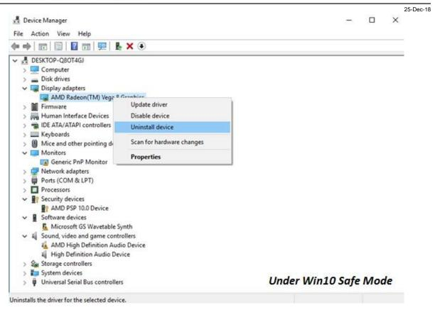
8. Check the box "Delete the driver software for this device" and click Uninstall.
