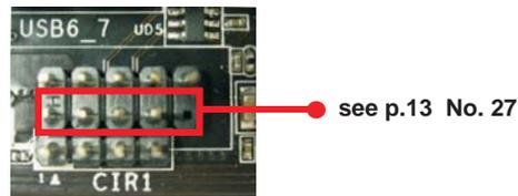
With ASRock XFast Charger feature, you can freely enjoy the quick charging convenience by installing the USB cable on these two ports.
