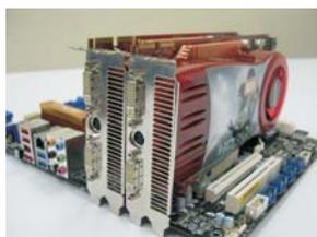
Step 3. Install one Radeon graphics card to PCIE6 slot. For the proper installation procedures, please refer to section “Expansion Slots”.
