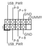
Besides two default USB 2.0 ports on the I/O panel, there are four USB 2.0 headers on this motherboard. Each USB 2.0 header can support two USB 2.0 ports. Please be noted that USB6 port supports ASRock XFast Charger. Please refer to page 40 for detailed information.
