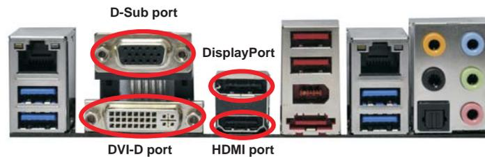
2. If you have installed onboard VGA driver from our support CD to your system already, you can freely enjoy the benefits of dual monitor function after your system boots. If you haven't installed onboard VGA driver yet, please install onboard VGA driver from our support CD to your system and restart your computer.
