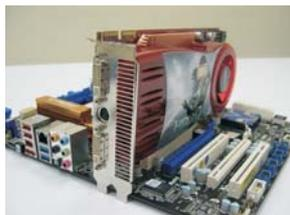
Step 2. Install one Radeon graphics card to PCIE4 slot. For the proper installation procedures, please refer to section “Expansion Slots”.
