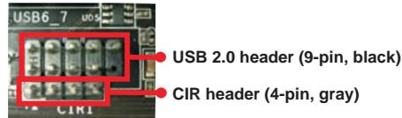
Step2. Connect the front USB cable to the USB 2.0 header (as below, pin 1-5) and the CIR header. Please make sure the wire assignments and the pin assignments are matched correctly.
