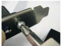
**Step 4** Put the rear USB 3.0 bracket into the chassis.
