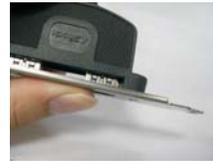
**Step 3** Screw the two screws into the rear USB 3.0 bracket.
