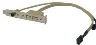
This PS/2 Mouse/Keyboard + USB 2.0 Bracket can support one PS2 Mouse/Keyboard port and two additional USB 2.0 ports besides the I/O panel. Please connect the 5-pin connector on the bracket cable to the PS2 header, and connect the 9-pin connector on the bracket cable to the USB 2.0 header (USB2\_3, USB4\_5, USB6\_7 or USB8\_9) and fasten the bracket to the chassis with screws.
