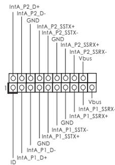
Besides four default USB 3.0 ports on the I/O panel, there is one USB 3.0 header on this motherboard. This USB 3.0 header can support two USB 3.0 ports.
