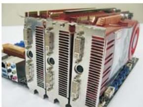
Step 4. Use one CrossFire™ Bridge to connect Radeon graphics cards on PCIE1 and PCIE4 slots, and use the other CrossFire™ Bridge to connect Radeon graphics cards on PCIE4 and PCIE6 slots. (CrossFire™ Bridge is provided with the graphics card you purchase, not bundled with this motherboard. Please refer to your graphics card vendor for details.)
