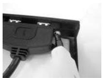
**Step 2** Put the USB 3.0 cable and the rear USB 3.0 bracket together.
