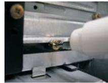
**Step 5** Plug the Front USB 3.0 cable into the USB 3.0 header (USB3\_5\_6) on the motherboard.
