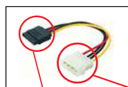
The SATA 15-pin power connector (Black) connect to SATA / SATAII / SATA3 HDD
