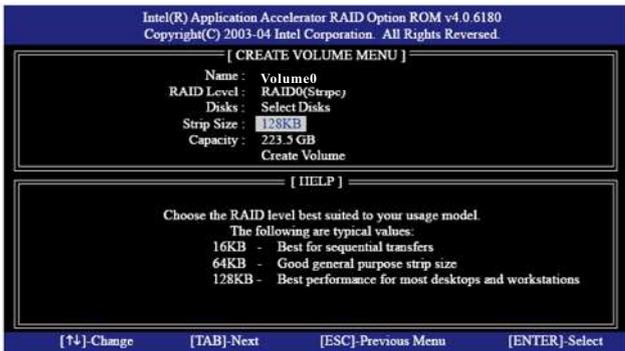
If you selected RAID 0 (Stripe), use the up or down keys to select the stripe size for your RAID 0 array then press <Enter>. The available values range from 8 KB to 128 KB. The default selection is 128 KB. The strip value should be chosen based on the planned drive usage.
