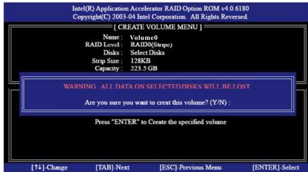
Press <Y> to complete the setup of RAID.
