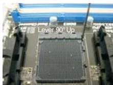
STEP 1: Lift Up The Socket Lever
