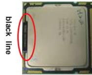
Step 3-2. Orient the CPU with the IHS (Integrated Heat Sink) up. Locate Pin1 and the two orientation key notches.
