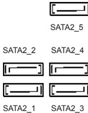
These five Serial ATA2 (SATA2) connectors support SATA data cables for internal storage devices. The current SATA2 interface allows up to 3.0 Gb/s data transfer rate.
