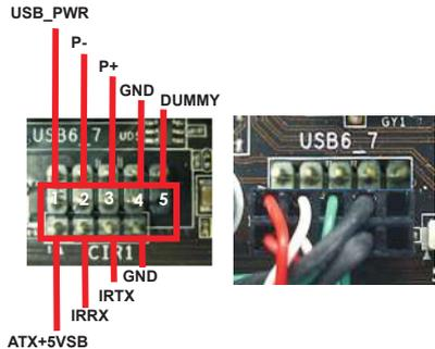
Step3. Install Multi-Angle CIR Receiver to the front USB port.
