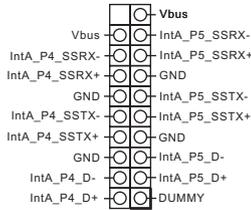
Besides two default USB 3.0 ports on the I/O panel, there is one USB 3.0 header on this motherboard. This USB 3.0 header can support two USB 3.0 ports.
