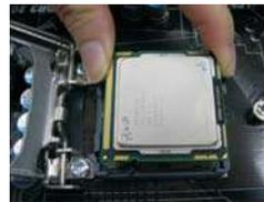
Step 3-4. Verify that the CPU is within the socket and properly mated to the orient keys.
