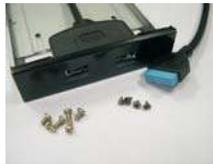
**Step 2** Screw the 2.5" HDD/SSD to the Front USB 3.0 Panel with four HDD screws.
