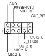
This is an interface for front panel audio cable that allows convenient connection and control of audio devices.
