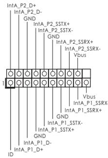
Besides two default USB 3.0 ports on the I/O panel, there is one USB 3.0 header on this motherboard. This USB 3.0 header can support two USB 3.0 ports.
