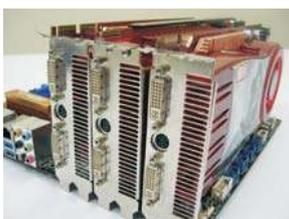
Step 4. Use one CrossFire™ Bridge to connect Radeon graphics cards on PCIE2 and PCIE4 slots, and use the other CrossFire™ Bridge to connect Radeon graphics cards on PCIE4 and PCIE5 slots. (CrossFire™ Bridge is provided with the graphics card you purchase, not bundled with this motherboard. Please refer to your graphics card vendor for details.)
