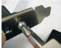
**Step 4** Put the rear USB 3.0 bracket into the chassis.
