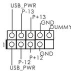
Besides six default USB 2.0 ports on the I/O panel, there are three USB 2.0 headers on this motherboard. Each USB 2.0 header can support two USB 2.0 ports.
