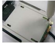
**Step 3** Install the Front USB 3.0 Panel into the 2.5" drive bay of the chassis.
