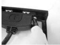
**Step 2** Put the USB 3.0 cable and the rear USB 3.0 bracket together.
