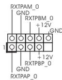
Besides one default IEEE 1394 port on the I/O panel, there is one IEEE 1394 header (FRONT\_1394) on this motherboard. This IEEE 1394 header can support one IEEE 1394 port.
