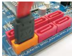
Connect the SATA data cable to the orange SATAII connector (SATAII_6 (Port5))
