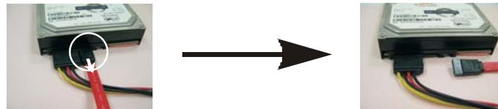
**Step 2** Unplug SATA 15-pin power cable connector (Black) from SATA / SATAII HDD side.
