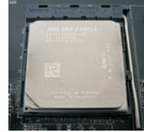
STEP 2 / STEP 3: Match The CPU Golden Triangle To The Socket Corner Small Triangle
