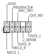
This is an interface for the front panel audio cable that allows convenient connection and control of audio devices.
