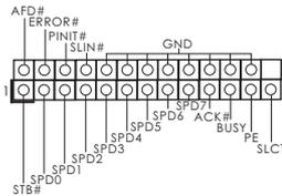
This is an interface for print port cable that allows convenient connection of printer devices.
