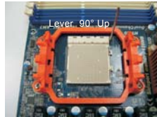
STEP 1: Lift Up The Socket Lever
