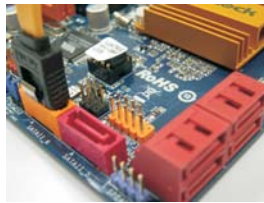
Connect the SATA data Cable to the SATAII connector (SATAII_6)
