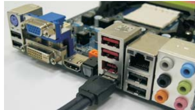
Connect the other end of the eSATAII device cable to eSATAII port of the I/O shield
