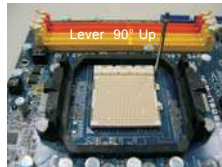
STEP 1: Lift Up The Socket Lever
