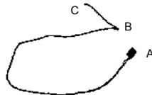
Please connect the black end (A) of HDMI\_SPDIF cable to the HDMI\_SPDIF header on the motherboard. Then connect the white end (B or C) of HDMI\_SPDIF cable to the HDMI\_SPDIF connector of HDMI VGA card.
