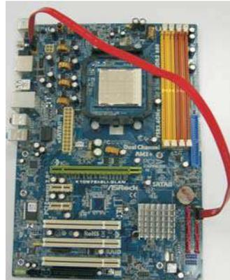
2. Use the eSATAII device cable to connect eSATAII device and the eSATAII port of the I/O shield according to the eSATAII connector that you connect the SATA data cable.
