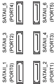
These six Serial ATAII (SATAII) connectors support SATA data cables for internal storage devices. The current SATAII interface allows up to 3.0 Gb/s data transfer rate.
