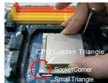
STEP 2 / STEP 3: Match The CPU Golden Triangle To The Socket Corner Small Triangle
