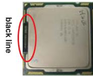
Step 3-2. Orient the CPU with IHS (Integrated Heat Sink) up. Locate Pin1 and the two orientation key notches.
