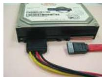
**Step 2** Unplug SATA 15-pin power cable connector (Black) from SATA / SATAII HDD side.
