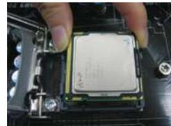
Step 3-4. Verify that the CPU is within the socket and properly mated to the orient keys.
