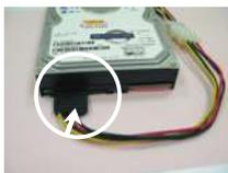
**Step 4** Connect SATA data cable to the SATA / SATA2 HDD.
