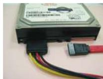
**Step 2** Unplug SATA 15-pin power cable connector (Black) from SATA / SATA2 HDD side.
