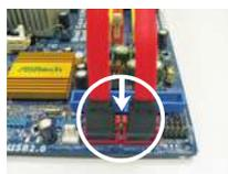
**Step 3** Connect SATA 15-pin power cable connector (Black) end to SATA / SATA2 HDD.
