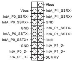
Besides two default USB 3.0 ports on the I/O panel, there is one USB 3.0 header on this motherboard. This USB 3.0 header can support two USB 3.0 ports.
