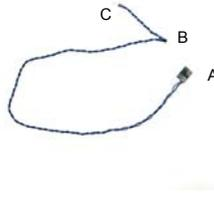
Please connect the black end (A) of HDMI\_SPDIF cable to the HDMI\_SPDIF header on the motherboard. Then connect the white end (B or C) of HDMI\_SPDIF cable to the HDMI\_SPDIF connector of HDMI VGA card.
