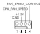
Please connect a CPU fan cable to this connector and match the black wire to the ground pin.
