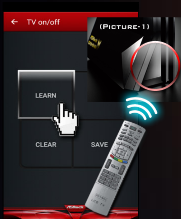
(Picture-1) Please put TV remote controller near to G10 IR Receiver Window within 10cm when you are in "LEARN" mode.
