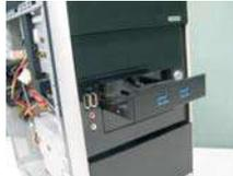
**Step 4** Screw the Front USB 3.0 Panel to the drive bay with six chassis screws.
