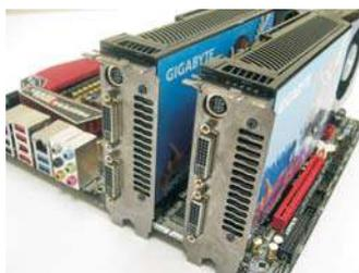
Step2. If required, connect the auxiliary power source to the PCI Express graphics cards.
