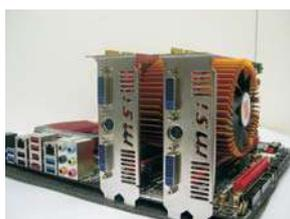
Step 3. Install one Radeon graphics card to PCIE5 slot. For the proper installation procedures, please refer to section “Expansion Slots”.
