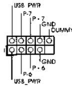
Besides four default USB 2.0 ports on the I/O panel, there are four USB 2.0 headers on this motherboard. Each USB 2.0 header can support two USB 2.0 ports.
