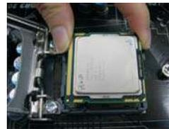
Step 3-4. Verify that the CPU is within the socket and properly mated to the orientation keys.
