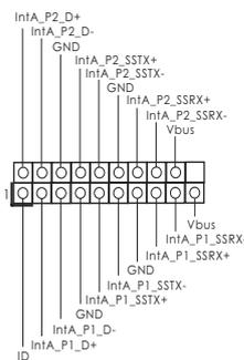
Besides four default USB 3.0 ports on the I/O panel, there is one USB 3.0 header on this motherboard. This USB 3.0 header can support two USB 3.0 ports.
