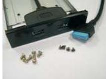
**Step 2** Screw the 2.5" HDD/SSD to the Front USB 3.0 Panel with four HDD screws.
