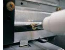
**Step 5** Plug the Front USB 3.0 cable into the USB 3.0 header (USB3\_2\_3) on the motherboard.
