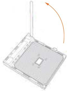
Step 2. Position the CPU directly above the socket such that the CPU corner with the golden triangle matches the socket corner with a small triangle.
