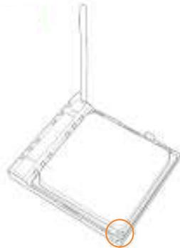
Step 4. When the CPU is in place, press it firmly on the socket while you push down the socket lever to secure the CPU. The lever clicks on the side tab to indicate that it is locked.
