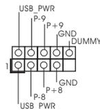
Besides four default USB 2.0 ports on the I/O panel, there are two USB 2.0 headers on this motherboard. Each USB 2.0 header can support two USB 2.0 ports.
