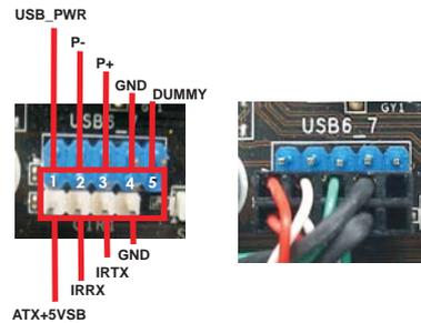
Step3. Install Multi-Angle CIR Receiver to the front USB port.
