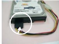
**Step 4** Connect SATA data cable to the SATA / SATAII / SATA3 HDD.
