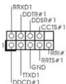
This COM1 header supports a serial port module.
