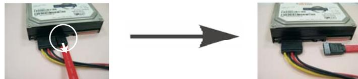
**Step 2** Unplug SATA 15-pin power cable connector (Black) from SATA / SATAII / SATA3 HDD side.
