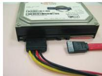
**Step 2** Unplug SATA 15-pin power cable connector (Black) from SATA / SATAII / SATA3 HDD side.
