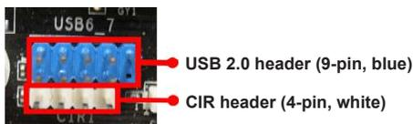
2. Connect the front USB cable to the USB 2.0 header (as below, pin 1-5) and the CIR header. Please make sure the wire assignments and the pin assignments are matched correctly.
