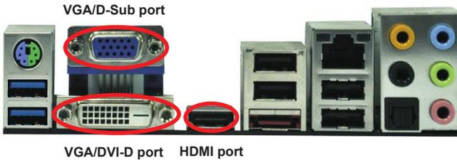
2. If you have installed onboard VGA driver from our support CD to your system already, you can freely enjoy the benefits of dual monitor function after your system boots. If you haven't installed onboard VGA driver yet, please install onboard VGA driver from our support CD to your system and restart your computer.
