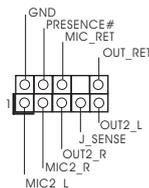
This is an interface for front panel audio cable that allows convenient connection and control of audio devices.
