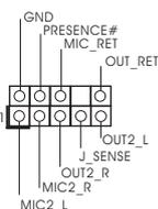
This is an interface for front panel audio cable that allows convenient connection and control of audio devices.
