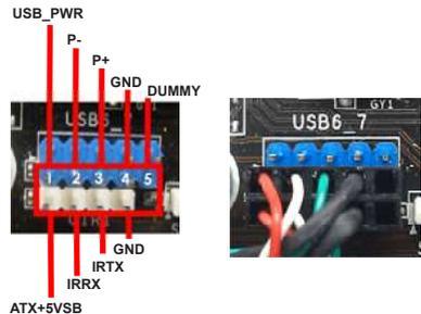
Step3. Install Multi-Angle CIR Receiver to the front USB port.
