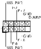
Besides the default USB 2.0 ports on the I/O panel, there are two USB 2.0 headers on this motherboard. Each USB 2.0 header can support two USB 2.0 ports.
