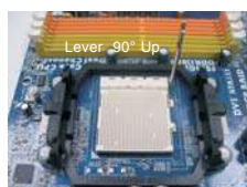
STEP 1: Lift Up The Socket Lever
