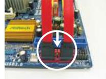
**Step 3** Connect SATA 15-pin power cable connector (Black) end to SATA3 HDD.
