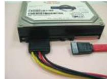
**Step 2** Unplug SATA 15-pin power cable connector (Black) from SATA3 HDD side.
