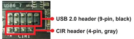
Step2. Connect the front USB cable to the USB 2.0 header (as below, pin 1-5) and the CIR header. Please make sure the wire assignments and the pin assignments are matched correctly.
