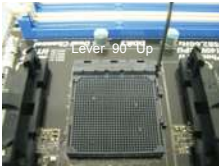
STEP 1: Lift Up The Socket Lever
