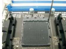
STEP 1: Lift Up The Socket Lever
