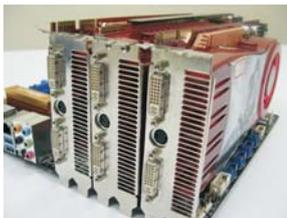
Step 4. Use one CrossFire™ Bridge to connect Radeon graphics cards on PCIE2 and PCIE3 slots, and use the other CrossFire™ Bridge to connect Radeon graphics cards on PCIE3 and PCIE4 slots. (CrossFire™ Bridge is provided with the graphics card you purchase, not bundled with this motherboard. Please refer to your graphics card vendor for details.)
