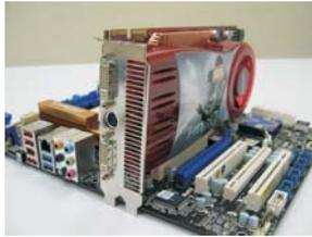
Step 2. Install one Radeon graphics card to PCIE3 slot. For the proper installation procedures, please refer to section “Expansion Slots”.
