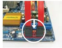
**Step 3** Connect SATA 15-pin power cable connector (Black) end to SATA3 HDD.
