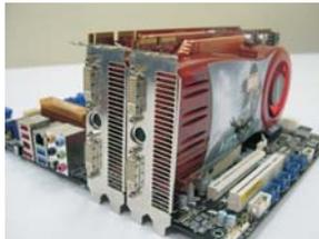
Step 3. Install one Radeon graphics card to PCIE4 slot. For the proper installation procedures, please refer to section “Expansion Slots”.
