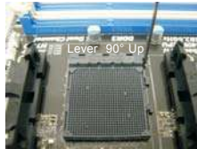
STEP 1: Lift Up The Socket Lever
