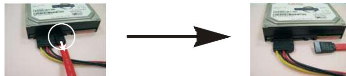
**Step 2** Unplug SATA 15-pin power cable connector (Black) from SATA3 HDD side.
