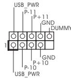
Besides eight default USB 2.0 ports on the I/O panel, there are three USB 2.0 headers on this motherboard. Each USB 2.0 header can support two USB 2.0 ports.
