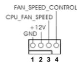
Please connect the CPU fan cable to this connector and match the black wire to the ground pin.
