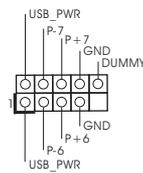
Besides four default USB 2.0 ports on the I/O panel, there are two USB 2.0 headers on this motherboard. Each USB 2.0 header can support two USB 2.0 ports.
