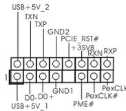
This header supports WiFi+AP function with ASRock WiFi-802.11g or WiFi-802.11n module, an easy-to-use wireless local area network (WLAN) adapter. It allows you to create a wireless environment and enjoy the convenience of wireless network connectivity.
