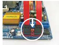
**Step 3** Connect SATA 15-pin power cable connector (Black) end to SATA / SATAII HDD.
