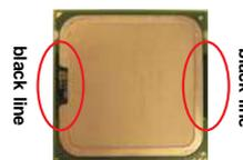
Step 2-2. Orient the CPU with IHS (Integrated Heat Sink) up. Locate Pin1 and the two orientation key notches.
