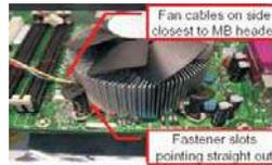
Step 3. Align fasteners with the motherboard throughholes.
