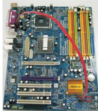
2. Use the eSATAII device cable to connect eSATAII device and the eSATAII port of the I/O shield.
