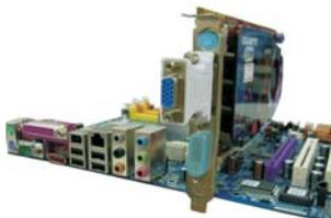
Step 3. Install the other Radeon graphics card to AGI Express slot (PCI Express x4). For the proper installation procedures, please refer to section “Expansion Slots”.
