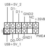
This header supports WiFi+AP function with ASRock WiFi-802.11g or WiFi-802.11n module, an easy-to-use wireless local area network (WLAN) adapter. It allows you to create a wireless environment and enjoy the convenience of wireless network connectivity.
