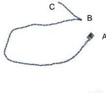
Please connect the black end (A) of HDMI\_SPDIF cable to the HDMI\_SPDIF header on the motherboard. Then connect the white end (B or C) of HDMI\_SPDIF cable to the HDMI\_SPDIF connector of HDMI VGA card.
