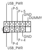
Besides four default USB 2.0 ports on the I/O panel, there is one USB 2.0 header on this motherboard. This USB 2.0 header can support two USB 2.0 ports.
